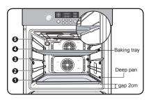
The baking tray, deep pan and wire grill should be inserted correctly into the side runners. When taking out the cooked foods from the oven, be careful of hot utensils and surfaces.
